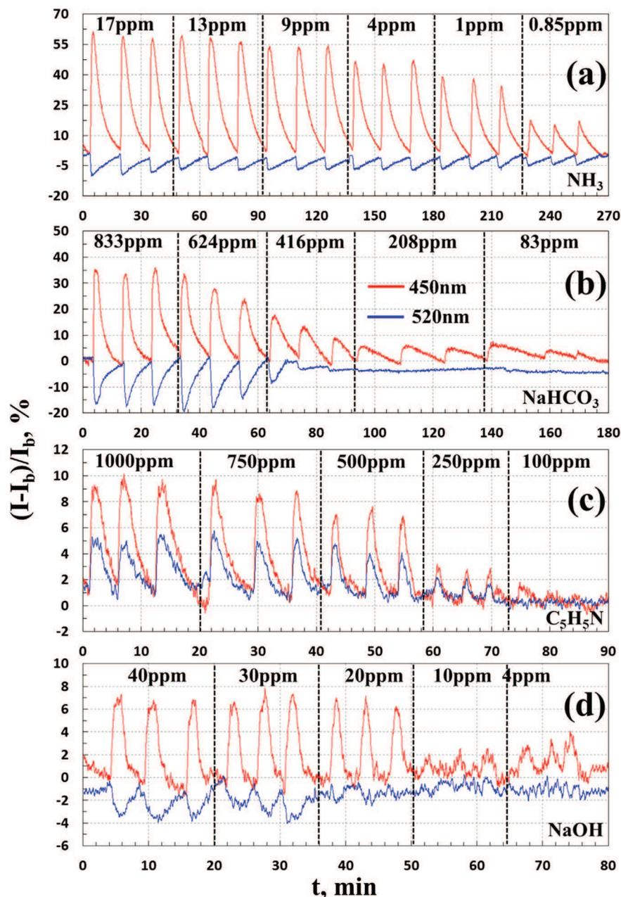
**Fig. 3.** Sensor response (transmittance normalized to baseline) to different concentrations of dissolved  $\text{NH}_3$  (a),  $\text{NaHCO}_3$  (b),  $\text{C}_5\text{H}_5\text{N}$  (c), and  $\text{NaOH}$  (d) at 450 nm (red color) and 520 nm (blue color).
