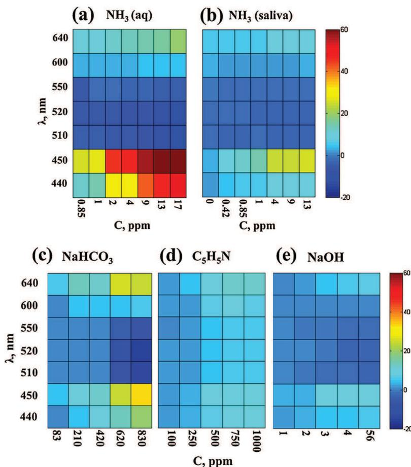
**Fig. 6.** Sensor response magnitude at a range of wavelengths for different concentrations of  $\text{NH}_3$  dissolved in deionized water (a) and diluted human saliva (b). Sensor responses to  $\text{NaHCO}_3$  (c),  $\text{C}_5\text{H}_5\text{N}$  (d) and  $\text{NaOH}$  (e) dissolved in deionized water are also shown.
