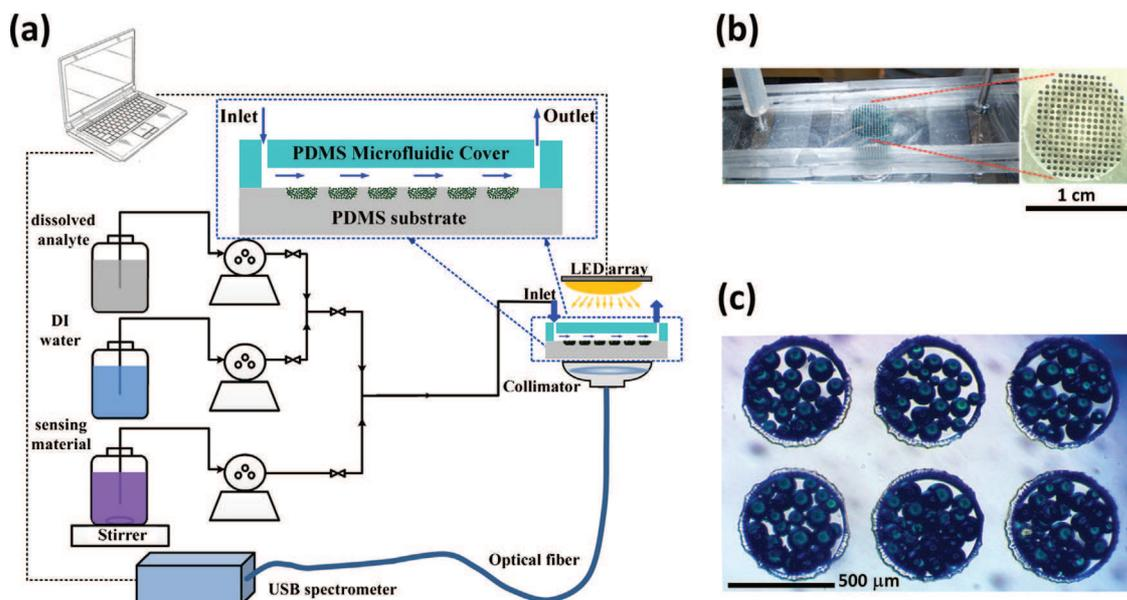
**Fig. 1.** (a) Schematic representation of the optical setup and flow system; (b) array of Zn(TPP)-doped microbeads embedded in the microfluidic device; and (c) a micrograph of Zn(TPP)-doped microbeads trapped inside microwells.
