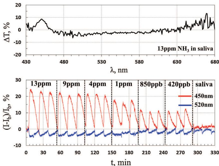
Fig. 4. Transmittance spectra recorded under the sensor exposure to 13 ppm NH<sub>3</sub> dissolved in diluted saliva (upper panel) and sensor response to different concentrations of NH<sub>3</sub> dissolved in diluted saliva at 450 nm (red color) and 520 nm (blue color).
