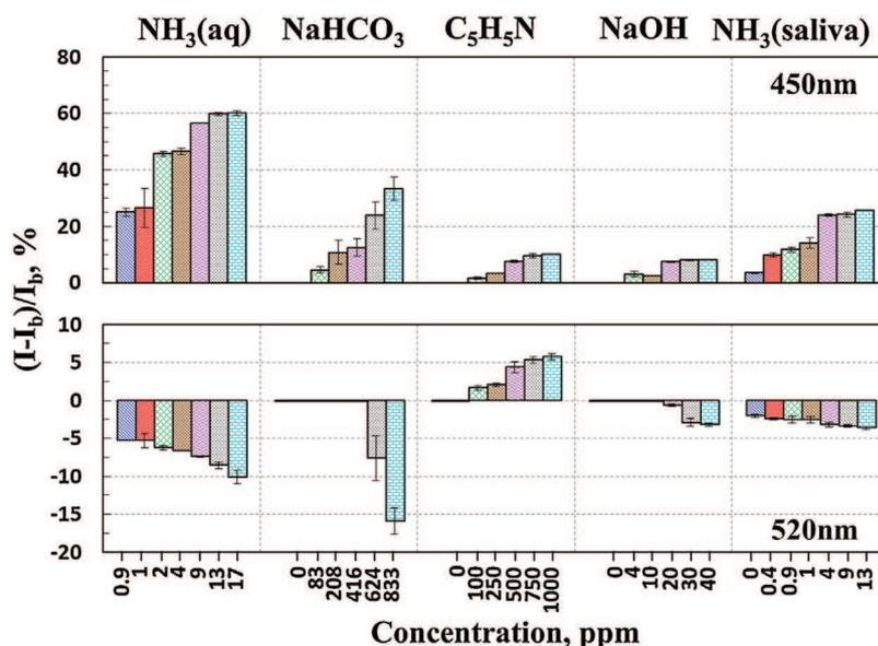
Fig. 5. Sensor response magnitude at 450 and 520 nm for different concentrations of NH<sub>3</sub>, NaHCO<sub>3</sub>, C<sub>5</sub>H<sub>5</sub>N, and NaOH dissolved in deionized water and of NH<sub>3</sub> dissolved in diluted human saliva. Error bars show standard deviation between three measurements.
