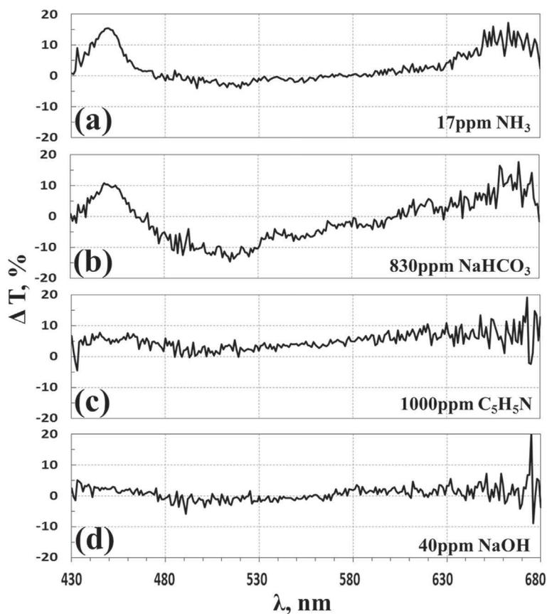
**Fig. 2.** Normalized transmittance spectra recorded under the sensor exposure to 17 ppm of  $\text{NH}_3$  (a), 833 ppm of  $\text{NaHCO}_3$  (b), 1000 ppm of  $\text{C}_5\text{H}_5\text{N}$  (d), and 40 ppm of  $\text{NaOH}$  (e) dissolved in deionized water.
